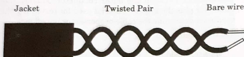
Fig. 1.15.2. Unshielded twisted pair cable.
